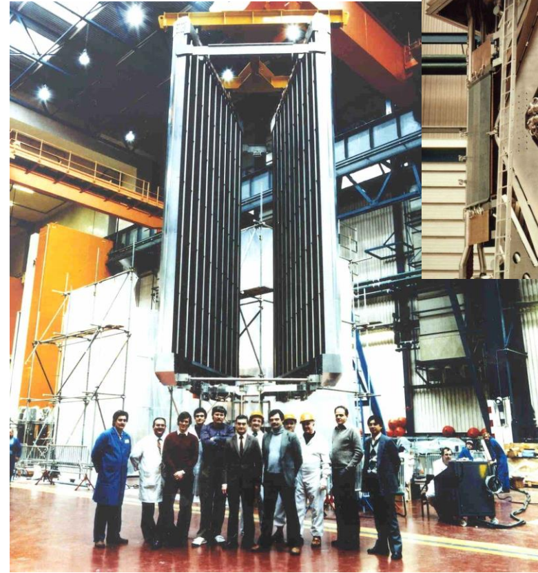
JET NB Injector cryopump
