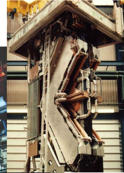
JET NB deflection magnet, residual ion dumps and calorimeter
